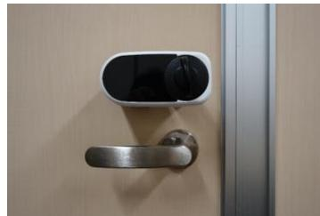
✓ When installed perpendicular to the thumb turn
